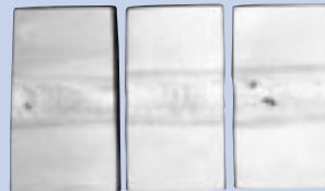
UNS N06022, (WNr. 2.4602) welded with INCO-WELD filler metal 686CPT.
