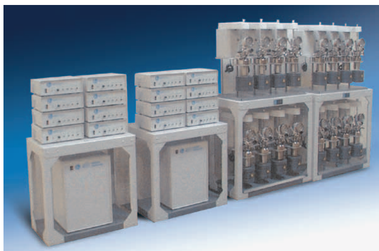
This custom order is set up to run sixteen reactors, two 4871 Process Controllers, with sixteen 4875 Power Controllers all through one PC.
