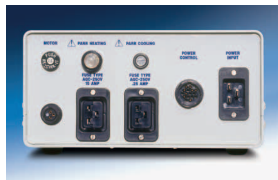
4875 Power Controller back panel for 230V model.
