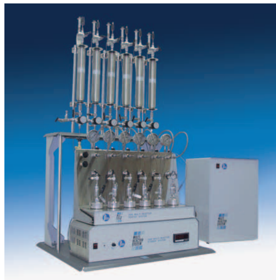
Series 5000 Multi Reactor System (MRS): a six station multi-reactor system. Each reactor is equipped with it's own constant pressure gas delivery system. The 4871 Controller maintains all of the important system parameters, including temperature and stirring speed, and records the gas consumption of each of the reactors.
