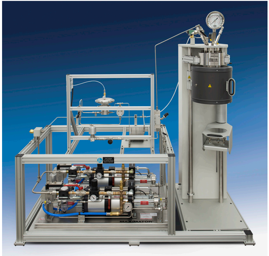
Automated Apparatus for Performing Hydrogen Induced Disbonding Tests
