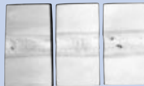
UNS N06022, (WNr. 2.4602) welded with INCO-WELD filler metal 686CPT.
