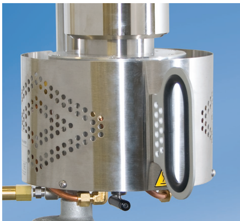
Aluminum Block Heater with Cooling Channel and Heat Shield for 1000 mL Vessel.
