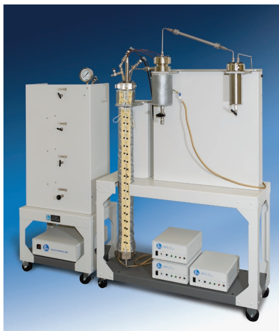
Parr Fluidized Bed Tubular Reactor with dual zone Mantle Heater.
