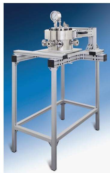
Pressure vessel with multiple 1-inch diameter windows installed.
