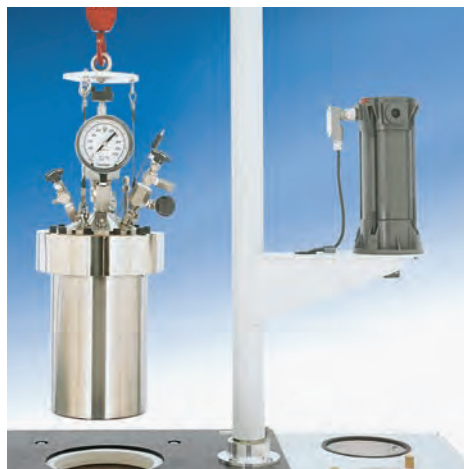
10 Liter Stirred Vessel removed from heater.
