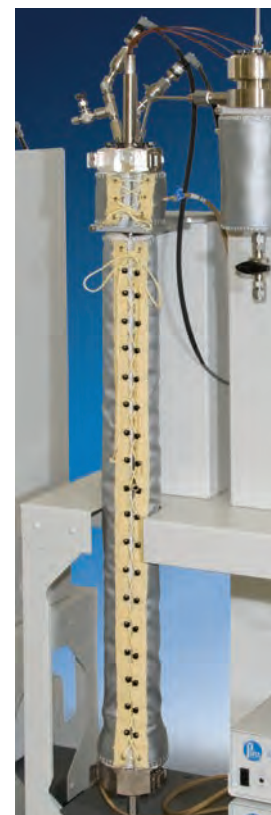
The Flexible Mantle Heater attaches in two pieces and provides even heating to the entire length of the reactor.
