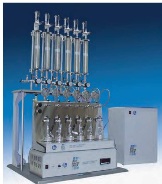
Series 5000 Multi Reactor System (MRS): a six station multi-reactor system. Each reactor is equipped with its own constant pressure gas delivery system. The 4871 Controller maintains all of the important system parameters, including temperature and stirring speed, and records the gas consumption of each of the reactors.
