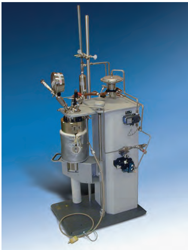
The supercritical fluid extraction system pictured left and diagramed above incorporates a 1.2 liter vessel rated for use at 3000 psig (200 bar) at temperatures to 300 °C. The system includes an automated inlet valve and an air-piloted back pressure regulator which is used to facilitate a controlled pressure release at the end of the test. The vessel is heated with a 1500W flexible mantle heater.
