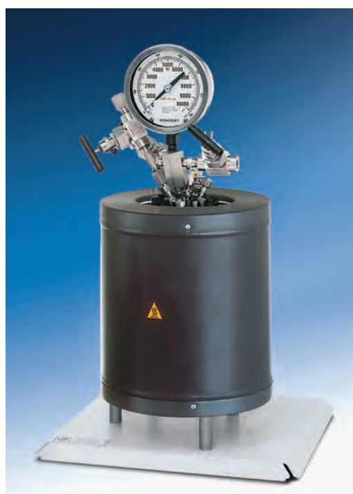
4652 Vessel with 4923 Heater.
