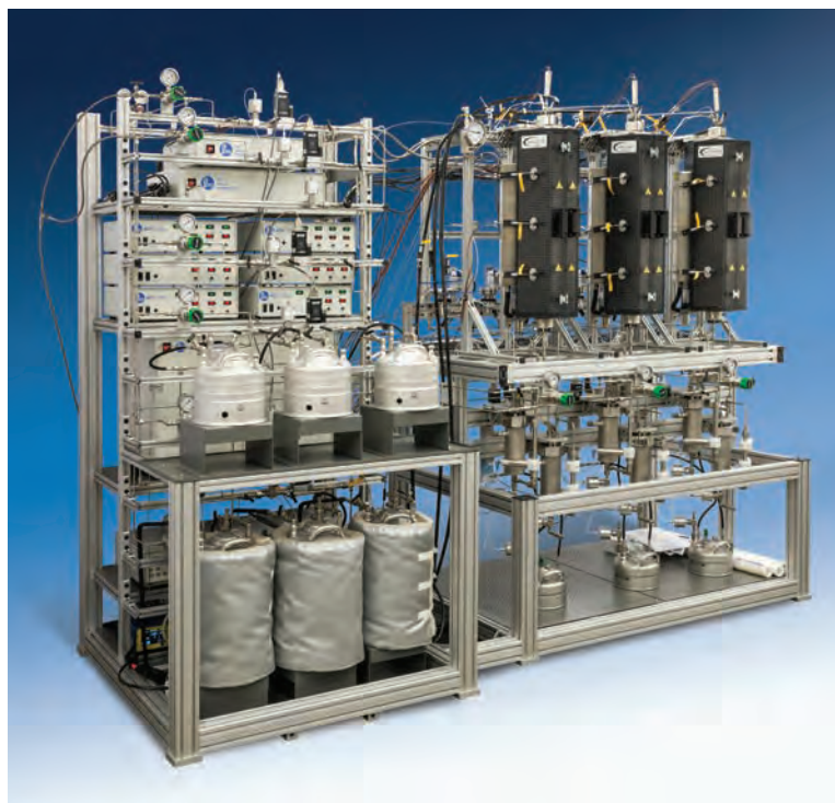
This system has three 250 mL reactors operating in parallel and controlled by a 4871 Process Controller with operator interface on a single PC. This system has weighed feed tanks and a two-stage pressure let down.
