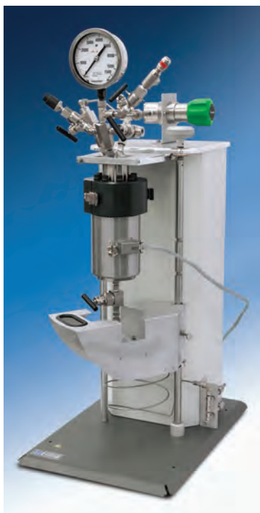
The batch supercritical extraction vessel pictured above is designed for use to 5000 psi (345 bar) at 350 °C. This 600 mL vessel was equipped with a liquid CO 2 pump capable of delivering up to 24 mL/min.
