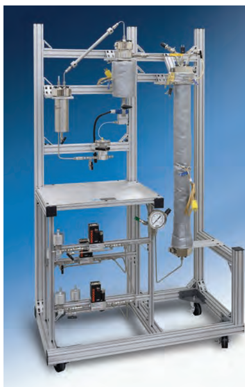
Flexible Mantle Heaters are wrapped around this 30"-long Fluidized Bed Reactor and the Cyclonic Separator to maintain temperatures to 350 °C. This system is also equipped with two gas feeds with automated shut-off valves, automated pressure control, and a Model 4871 Process Controller (not shown).
