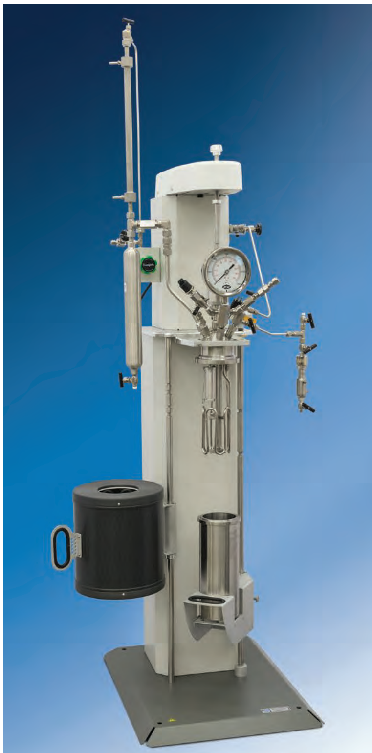
4534 Floor Stand Reactor, 2000 mL, Fixed Head, with Spiral Cooling Coil and Liquid Charging Pipette, in the open position, and a 4848 Controller with optional Expansion Modules.
