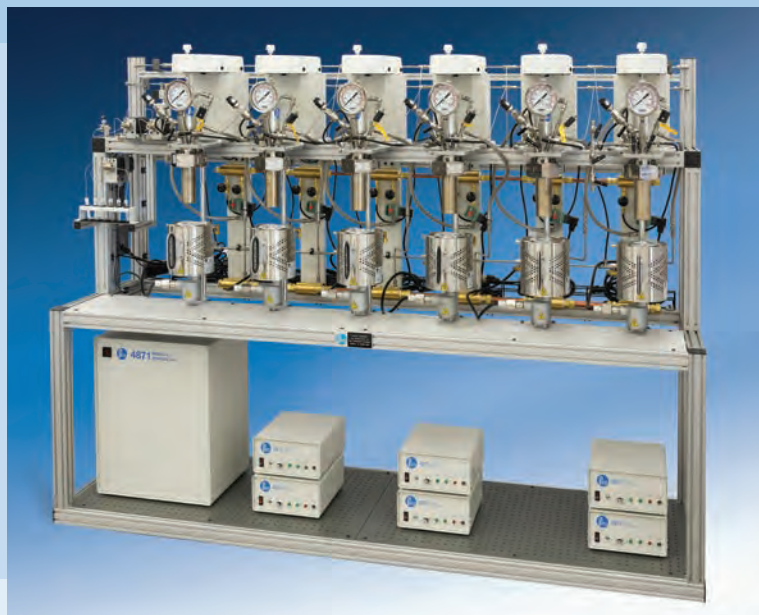
Six reactor 4590-based multi-reactor with automated sampling. See page 73.
